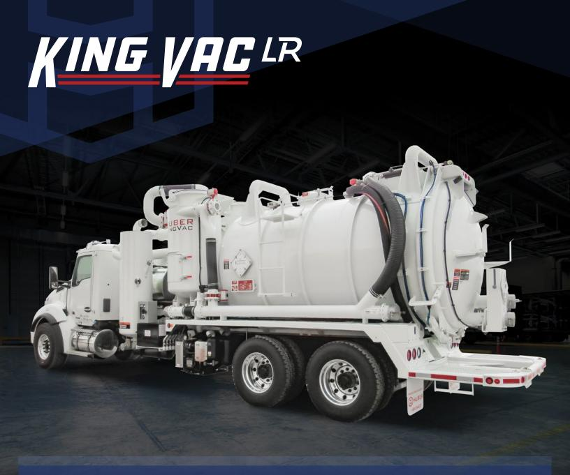
The Huber King Vac has been a leader since 1986 in the Liquid Ring vacuum industry with a 4,100 CFM pump. With its unmatched power and versatility, it can handle jobs that require deep vacuum or high air conveyance. This unit also allows the operator to clean out the filtration cyclones without shutting down allowing for maximum productivity. Scan the QR code or go to keithhuber.com to build your Huber unit today.
